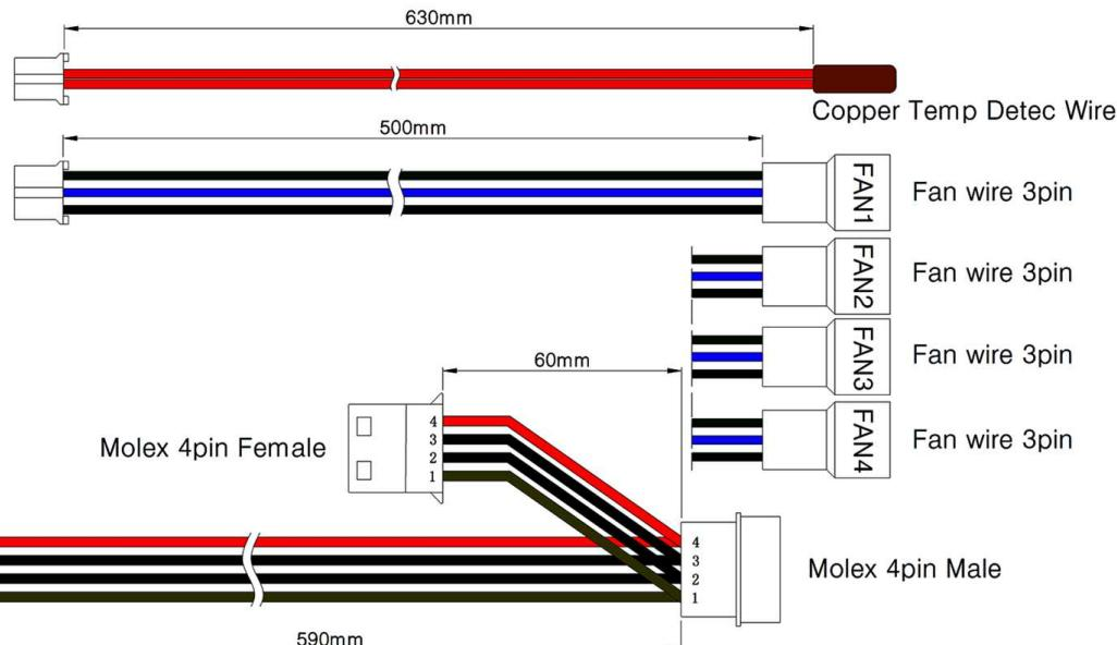
Default: all fans automatically activated or stopped if system temperature higher or lower than 38 degree-C
